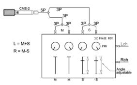
as L ch. and R ch. The angle between L and R can also be varied by the adjustment of the S ch. fader volume. When levels of M and S are the same, the stereophonic angle is  $127^{\circ}$ .
